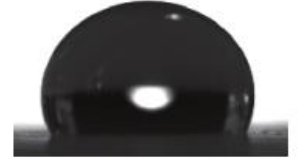
Water droplet on painted surface with SurfaPaint Aqua X Contact angle: 126°
