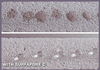
The results of water being dropped on a porous surface coats with Enviro SurfaPore C (bottom) as opposed to uncoated (top). The water simply sits on top of the surface as it is unable to penetrate into the pores.
