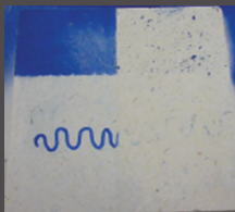
Anti-graffiti effect on porous surface. Right side cleaned under hot water without scrubbing.
